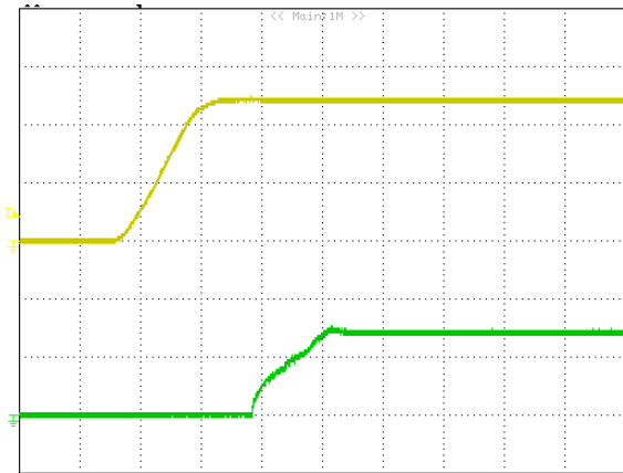
Figure 11: Turn on delay time at 12Vin, 0.8V/30A out. (Green : VOUT, 0.5V/div, Yellow: VIN, 5V/div. 1mS/div)
