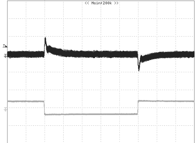
Figure 9: Output voltage response to step-change in load current (75%-50%-75% of I_o , max; di/dt = 2.5A/\mu s ). Load cap: 330\mu F , 35m\Omega ESR solid electrolytic capacitor and 1\mu F ceramic capacitor. Top Trace: V_{out} (100mV/div, 200us/div), Bottom Trace: I_{out} (5A/div). Scope measurement should be made using a BNC cable (length shorter than 20 inches). Position the load between 51 mm to 76 mm (2 inches to 3 inches) from the module
