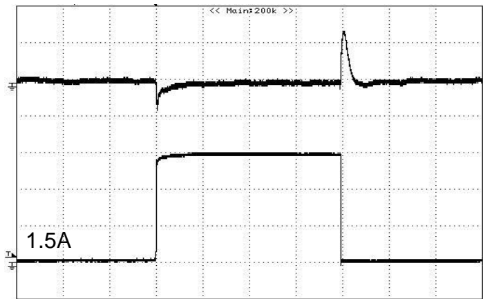
Figure 21: Typical transient response to step load change at 10A/μS between 50% and 100% load, at 12Vin, 0.59V out; CH2: VOUT(0.1V/div), CH4: Iout (0.5A/div), 100uS/div
